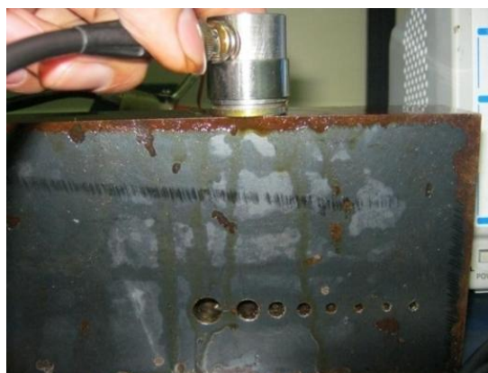
Figure 5. Schematic of the DAC calibration block.
