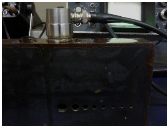
Figure 6. Actual DAC calibration block.
