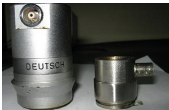
Figure 14. Comparison between (A) the factory-made probe and (B) the fabricated probe.
