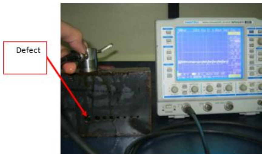
Figure 13. Echo pulse at a flaw depth of 100 mm.
