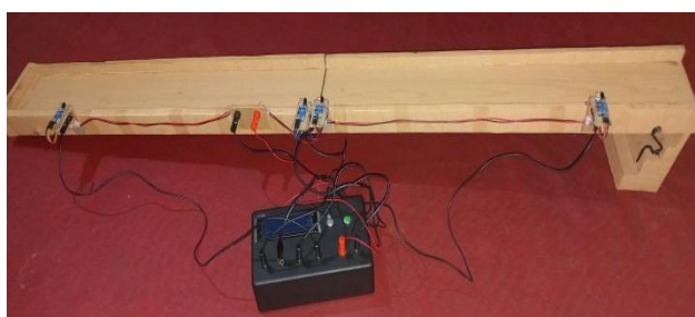
Figure 2. Hardware configuration of the automatic-timer-based UALM teaching aid
