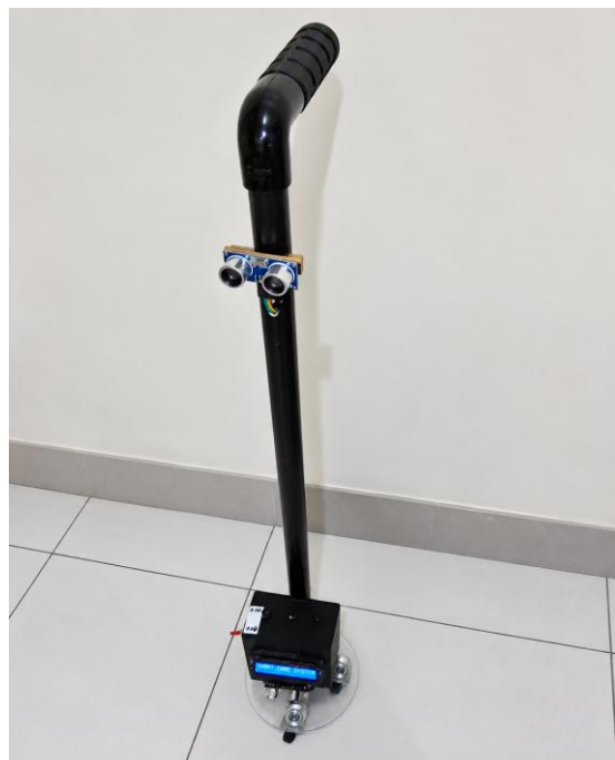
Figure 2. Developed smart cane prototype.
