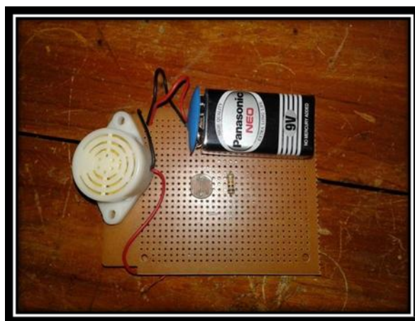
Figure 1. Design Scheme of the Simple Light Sensor Implementation
