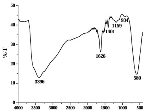
Figure 3. FTIR spectrum of SnO<sub>2</sub> Nanoparticles
