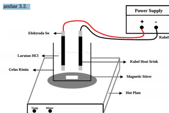
Figure 2. Schematic of Electrolysis Cell for Synthesis of SnO<sub>2</sub> Nanoparticles
