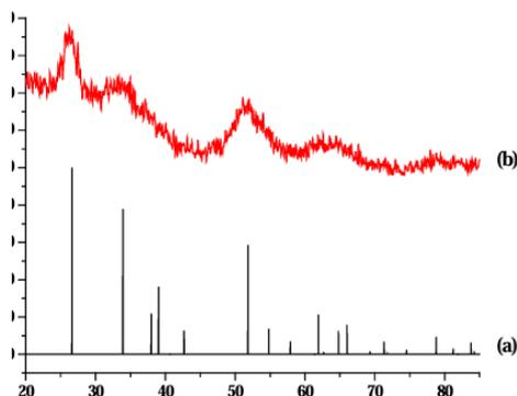
Figure 4. XRD spectra of (a) Standard SnO<sub>2</sub> (b) SnO<sub>2</sub> Synthesized by Electrochemical Method
