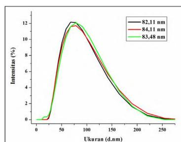
Figure 6. Distribution of Size of Analysis Results of Zeta Sizer Instrument during Electrolysis with HCl Concentration of 0.06 M at Potential of 60 Volts
