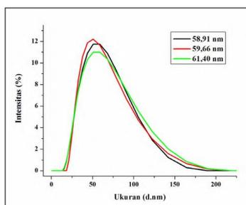
Figure 5. Distribution of Size of Analysis Results of Zeta Sizer Instrument during Electrolysis with HCl Concentration of 0.02 M at Potential of 60 Volts
