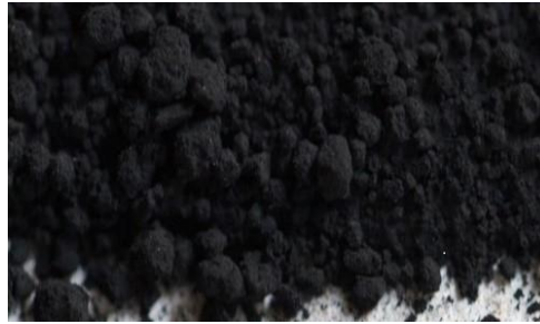
Figure 1. Waste tyre powder from the pyrolysis process
