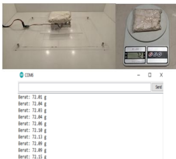
Figure 12. Loadcell Sensor Testing
