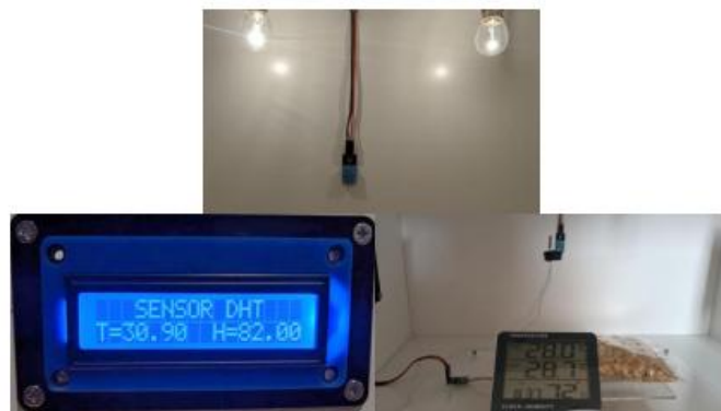
Figure 11. DHT11 Sensor Testing
