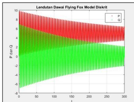
Figure 1. Simulation of the Flying Fox String Deflection Discrete System: initial values for  $P(0) = 0, Q(0) = 0, \delta_1 = 1/100, m_b = 50, \text{ and } m_d = 50$
