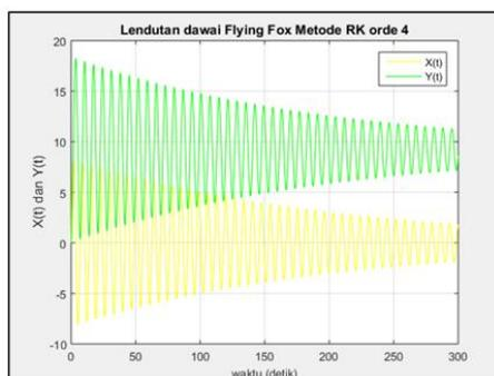
Figure 2. Simulation I of the Flying Fox String Deflection Continuous System: initial values for  $P(0) = 0, Q(0) = 0, \delta_1 = 1/100, m_b = 50, \text{ and } m_d = 50$
