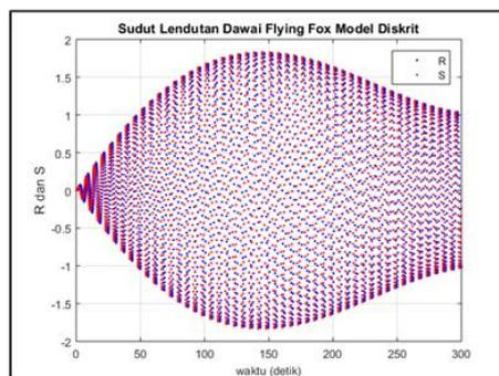
Figure 3. Simulation of the Flying Fox String Deflection Discrete System: initial values for  $R(0) = 0, S(0) = 0, \delta_2 = 1/100, m_b = 50, \text{ and } m_d = 50$
